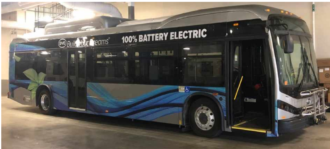
Figure 1 Saskatoon's electric test bus (model K9MC, assembled in California by the Chinese manufacturer BYD)
